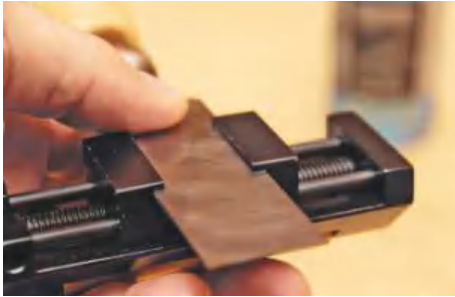
▲ As the guide is tightened, the blade is lifted until it is secured against the side tabs
